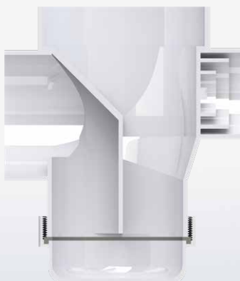
Gully Body Sectional View
