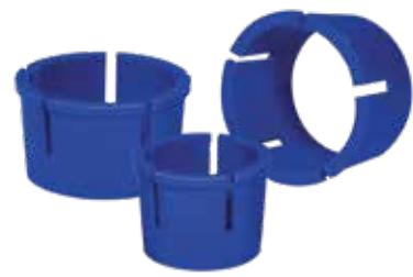
Smart Inserts are compact, cylindrical elements engineered for insertion into the inner walls of HDPE (High Density Polyethylene) pipes as part of the installation process. They find their primary application in pipes with wall thicknesses measuring less than 3.5mm, specifically within the nominal diameter range of 20mm to 32mm (Please consult Table 2 for specific details).
