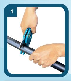
**Step 1**Cut the HDPE pipe using pipe cutter to the required length.
